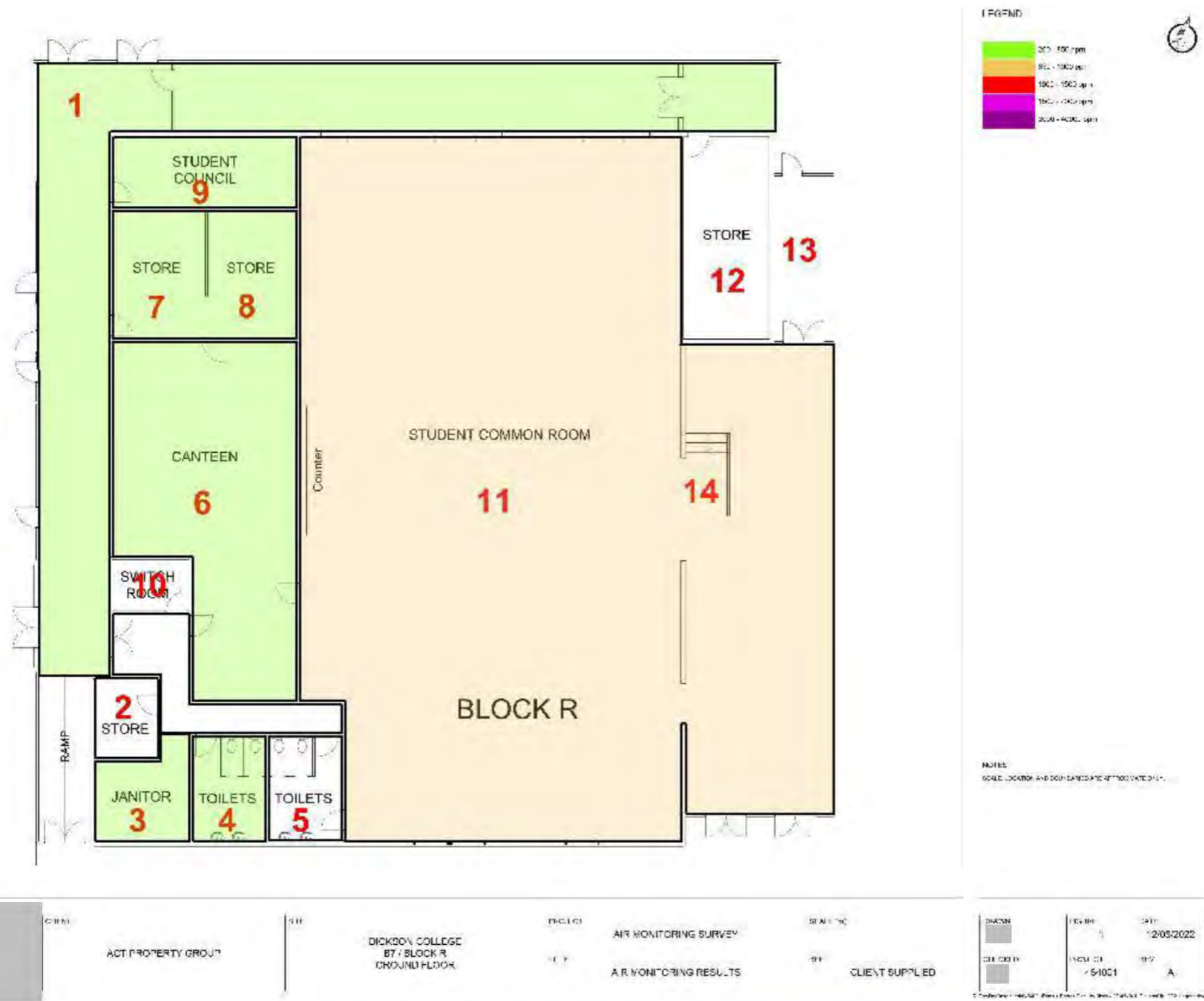
Figure 144: Block R (B7) Ground Floor Carbon Dioxide Averaged School Hour Levels
