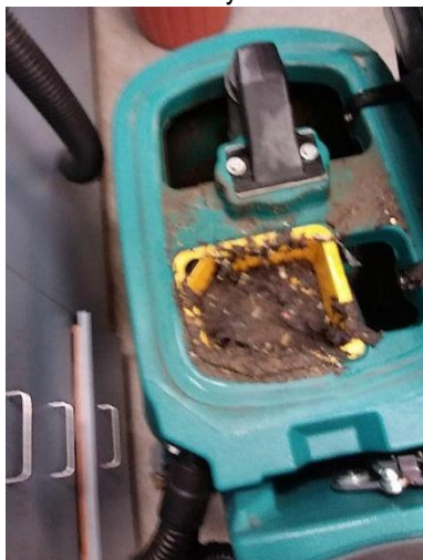
Figure 30: Scrubber/Dryer Recovery tank Alfred Deakin High
