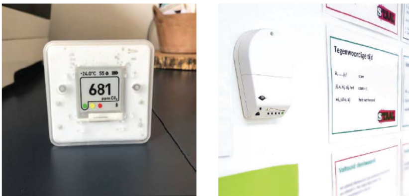
Figure 2. Examples of CO 2 monitors with traffic light indicator showing the indoor air quality.
