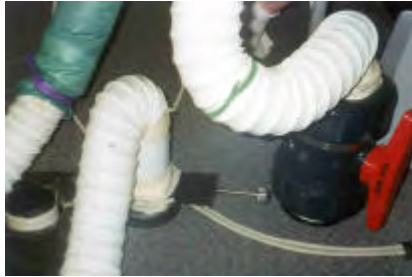
Figure 4.2 Local cold- and warm-air supplies (valves, flexible warm and cold air ducts to connect to air-sleeves)
