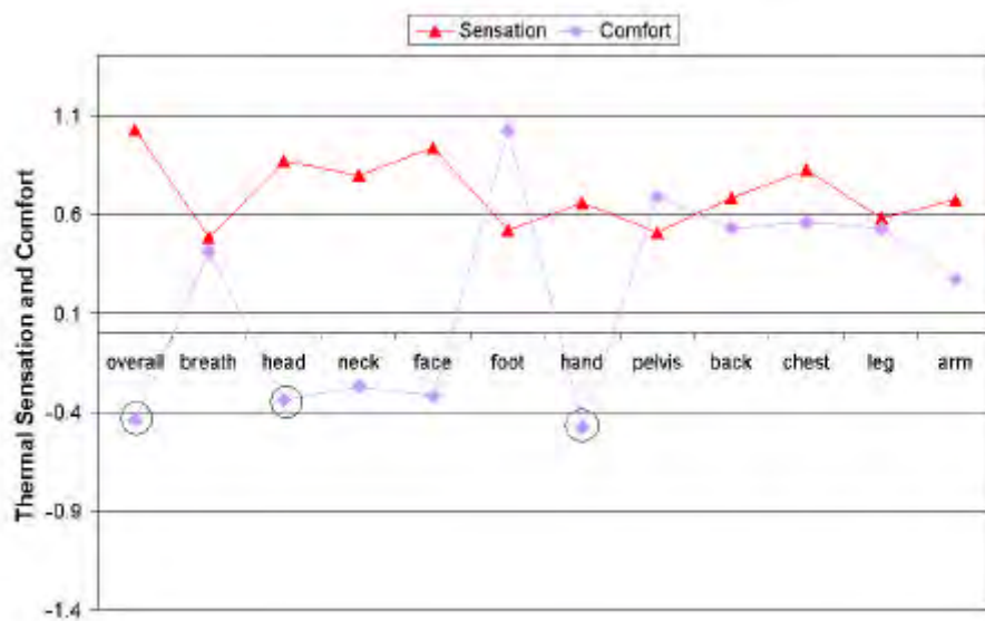
Figure 6.54 Validation of overall comfort model for UC Berkeley chamber experiment data in slightly warm environment (overall sensation near 1, 3 tests)
